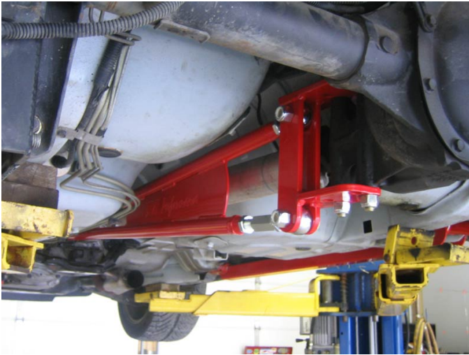
Image 3- Rear Torque Arm Mount Bolted in Place
