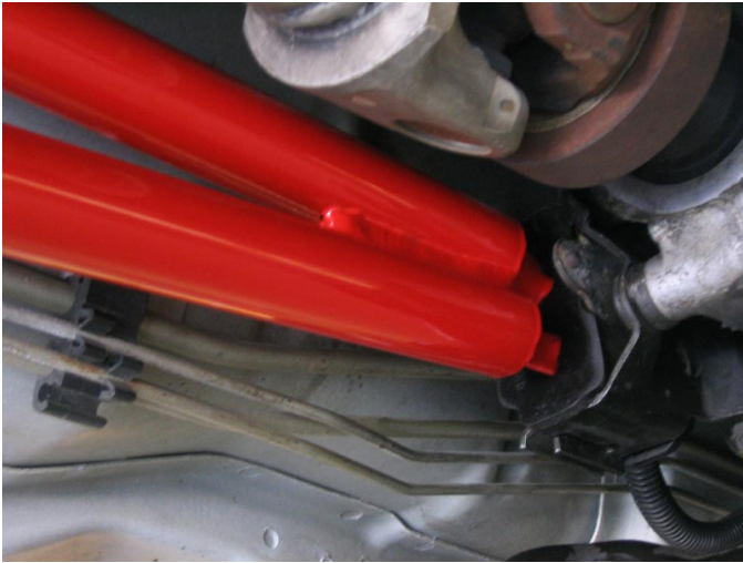
Image 3- Rear Torque Arm Mount Bolted in Place
