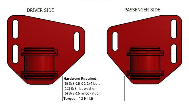
5. Install Engine side mounts. Final torque fasteners at this time. 45 ft lb.
