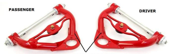
Note tubing welded flat to plate to determine a-arm side.
