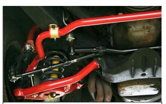
Check Sway Bar orientation at ride height. If bar is installed correctly, the bar ends should be level. If bar is installed upside down, the bar ends will run uphill.
