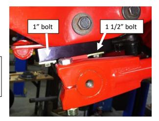
10. Install collar clamps onto the sway bar to eliminate side to side movement. These should be installed on the inside of the bushings, with a small (1/16") gap. Ensure to center the bar from side to side.
