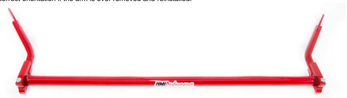
7. Using the supplied  $3/8-16 \times 2 \frac{1}{2}$ " gr.5 (3 lines on bolt head) bolts, install sway bar arm clamp bolts from the top side down. Use a washer and 3/8-16 nylock to secure.
