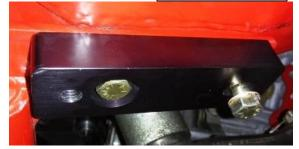
6. Preassemble Sway bar arms onto the spline bar before installing in car. The splined arms must be clocked the same, so that both ends will sit flat when sitting on a table or floor. If one arm is off, simply remove, clock 1 spline or more, then reinstall.
