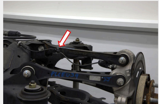
Figure 2: Wheel Speed Sensor Clips
