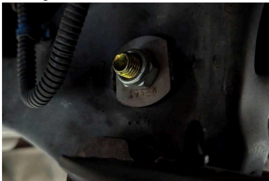
Figure 6: Eccentric Nut Delete Washer
