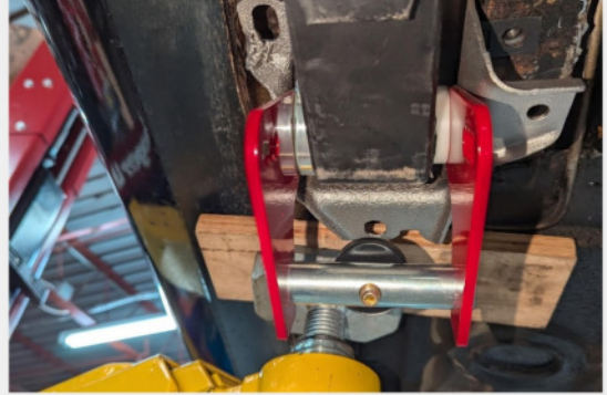
Fig 1. Remove three bolts holding the perch in place
