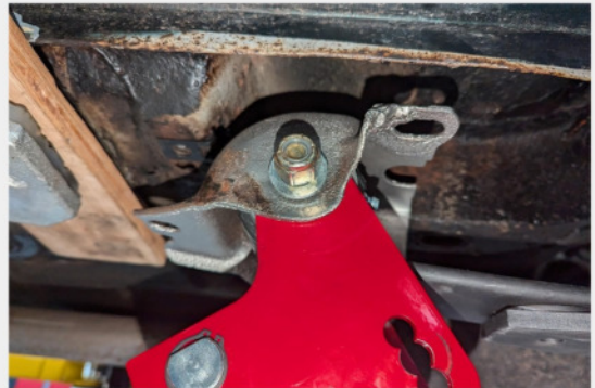
Fig 2. Remove leaf spring bolt .
