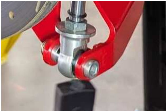
Fig 10: Spacer orientation in lower mount
