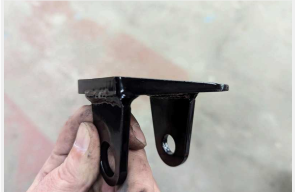
Figure 6: Passenger side mount is tapered
