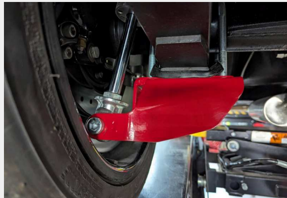
Figure 4: Install lower leaf spring plates.
