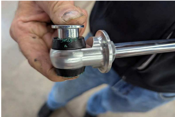
Fig 9: Bushing install in Viking Shocks Grease the bushing Before sliding the spacers into place.
