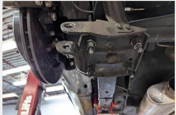
Figure 3: Remove U bolts and lower leaf spring plates.
