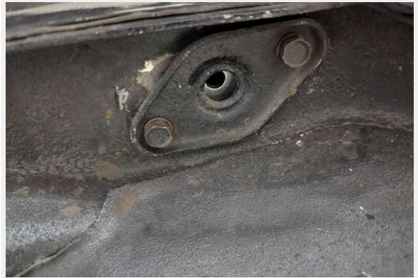
Figure 5: Shock Mount removal
