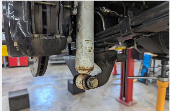
Figure 2: Remove the lower shock bolts.
