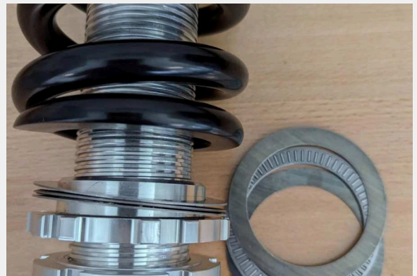
Figure 13: Perch Nuts, Thrust Bearing installed
