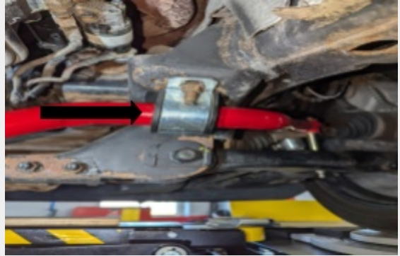
Fig 1. Apply Grease to the Bushing Mating Surface.
