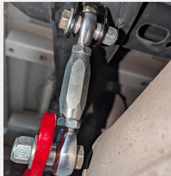
Figure 3: Sway Bar end links Installed
