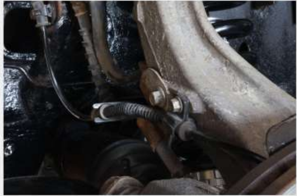
Figure 1: ABS Cable Removal
