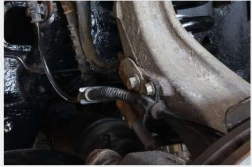
Figure 1: ABS Cable Removal
