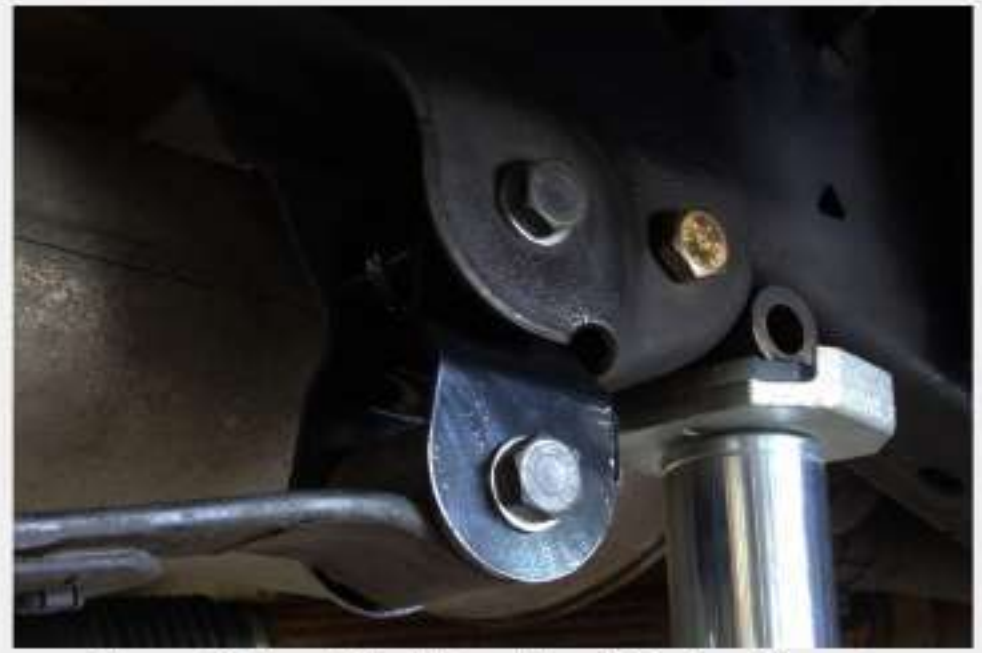
Figure 27: Installed Front Leaf Spring Mount
