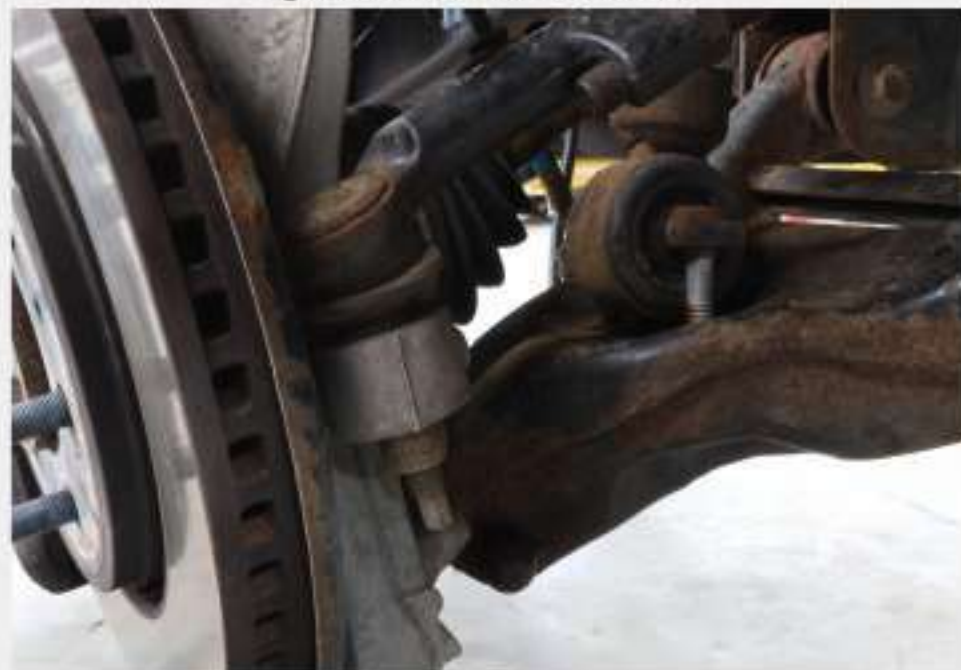
Figure 4: Tie rod end removal
