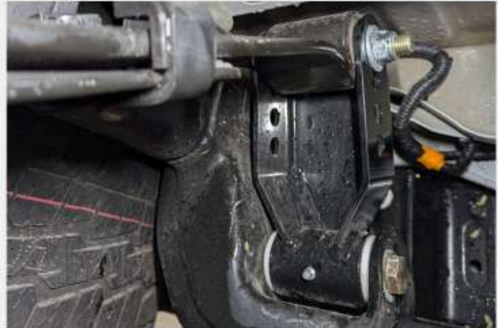
Figure 28: Installed Adjustable Leaf Spring Shackle
