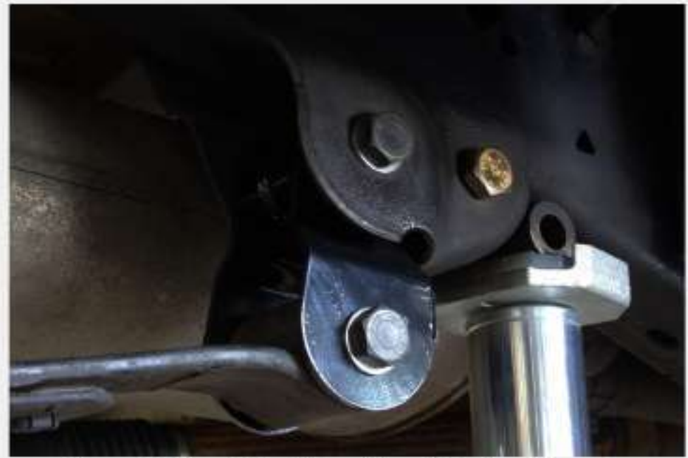
Figure 27: Installed Front Leaf Spring Mount
