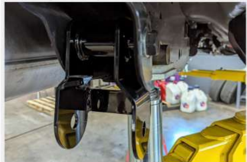
Figure 25: Installed Front Leaf Spring Mount
