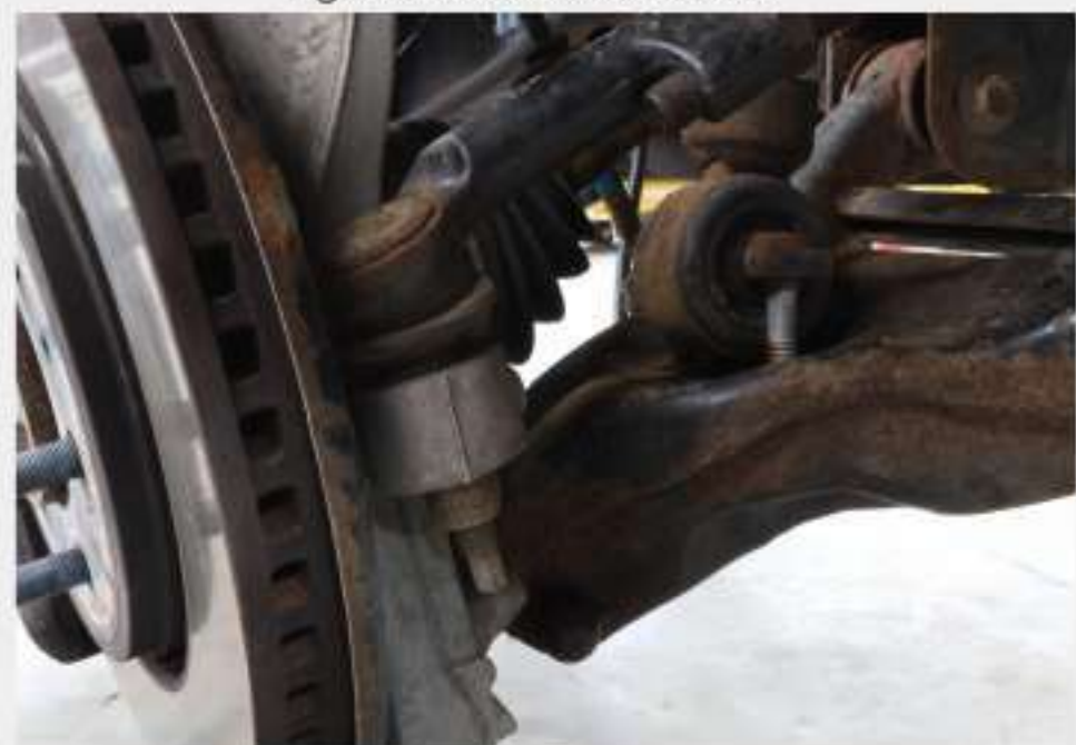
Figure 4: Tie rod end removal
