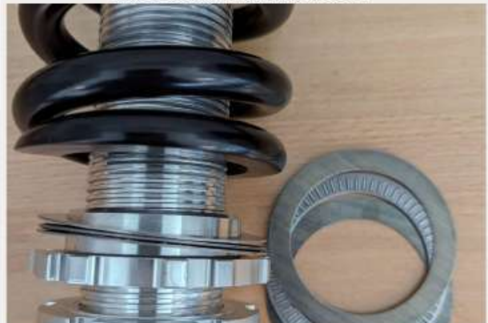
Figure 10: Perch Nuts, Thrust Bearing installed
