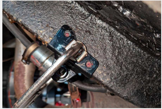
Fig 5: Lock bracket to frame and mark holes.
