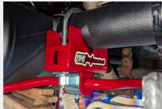
Fig 3. Install sway bar clamps to the axle.
