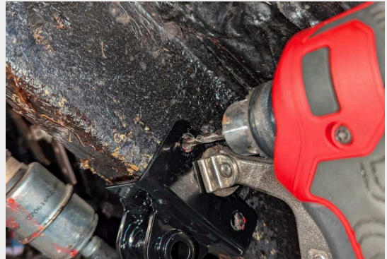
Fig 6: Smaller pilot hole first.
